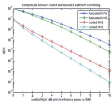
Fig.4 comparison between ber of oc and ldpc-oc system
